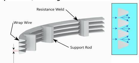
Monoflex Stainless Screens use v-shaped wedge wire wound and resistance welded around a profile of internal support rods.
